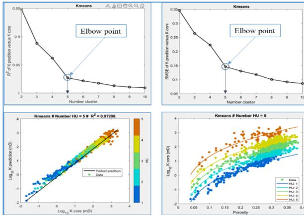
Figure 3.4: Result of HFU's number selection and the HFU classification method based on K-means method
