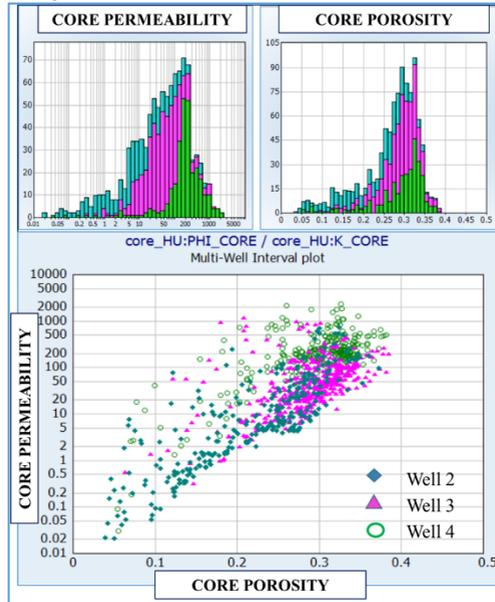
Figure 1.8: Porosity-Permeability Relationship from Core Sample Analysis Results in the CX Field.
