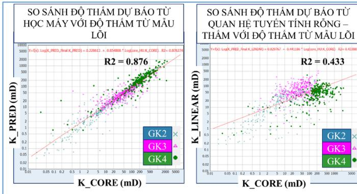
Figure 4.17: Comparison permeability prediction results with ML method (left) and with traditional linear regression method (right)
