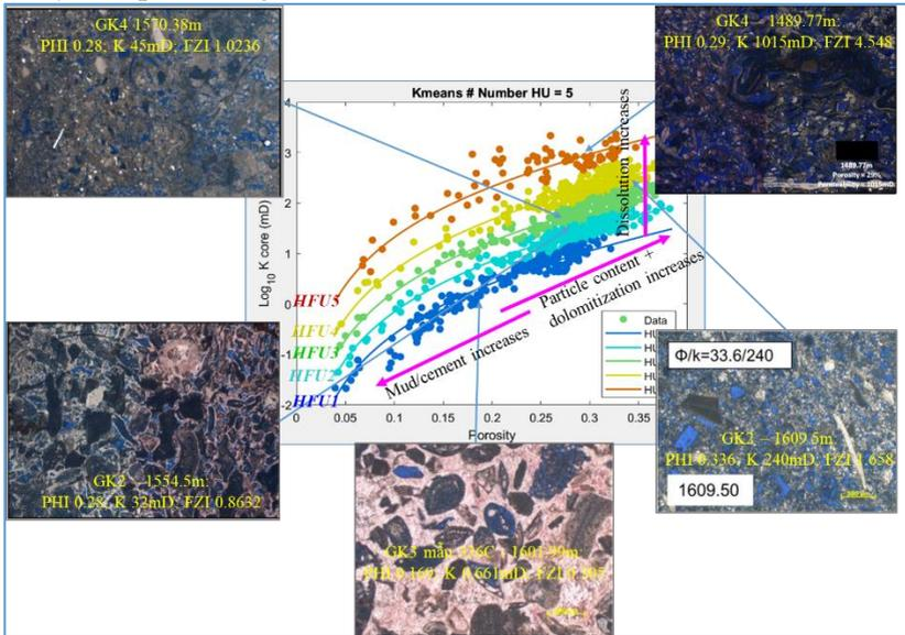
Figure 3.9: Representative thin section analyses for the classified HFUs at the CX wells.
