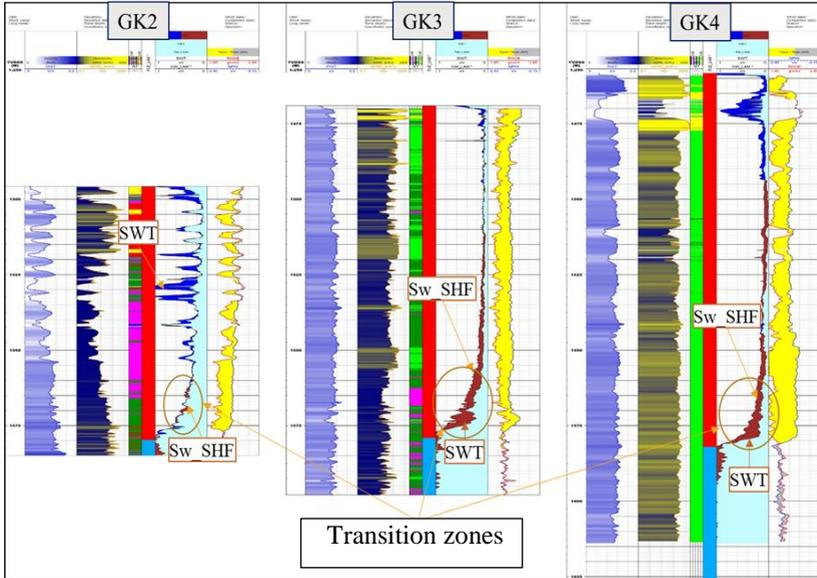
Hình 5.12: Sw estimation result using SHF model built for 5 HFUs
